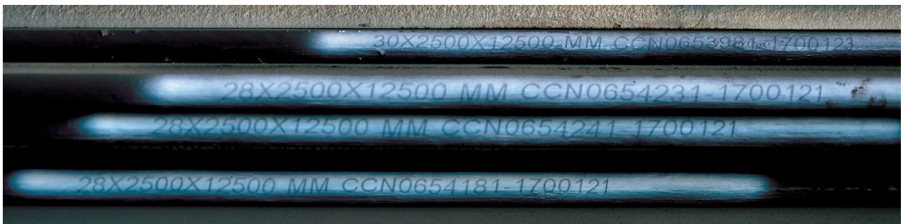
Marking on Plate Mill Plates from New Plate Mill of RSP
